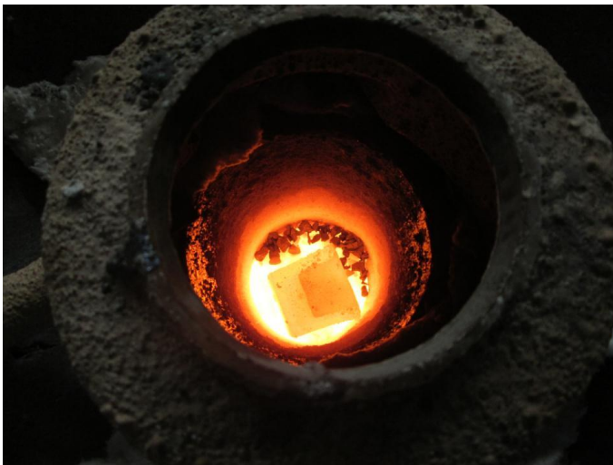
Dissolution of NbC-Fe during melting down of the metallic charge in an induction furnace.
