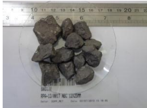
Medium particle size NbC-Fe (12-25 mm).
