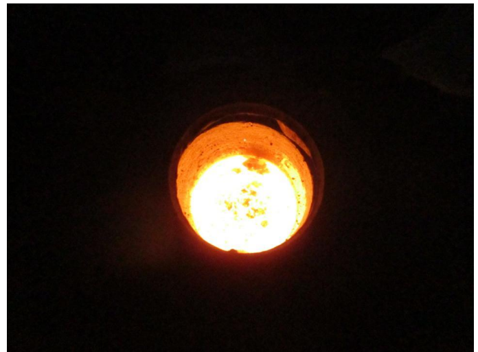
Dissolution of NbC-Fe by addition to the bath after the melting down of the metallic charge.
